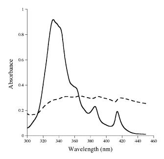
**Figure 2.** Spectroscopy of AMB samples. UV/Visible absorbance spectra of ABLC (dashed line) and apoA-I solubilized ABLC (solid line). Samples (12.4  $\mu$ g AMB/mL) were scanned from 300 to 450 nm.
