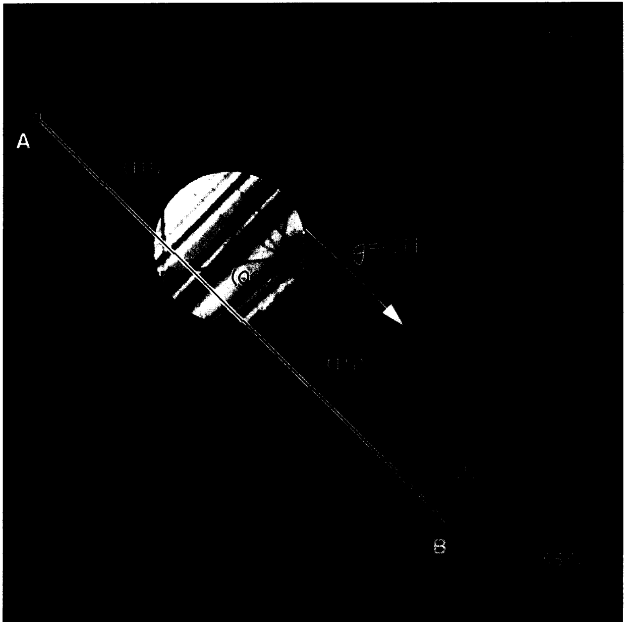
Fig. 5. Elastic CBED pattern taken from a single crystal of silicon using a systematic diffraction geometry. The pattern was obtained using a Philips CM200/FEG and GIF system. The probe size used for obtaining this CBED pattern was 14 Å, the energy window was 10 eV and the primary beam energy was 196.15 keV.
